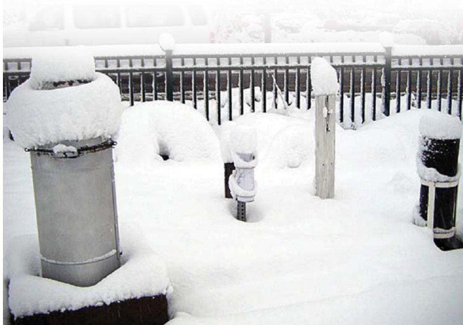
Figure 1. Most precipitation gauges do not measure snow very accurately. Courtesy of Wendy Ryan, Fort Collins weather station
