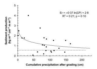
**Figure 11.** Relationship between sediment production (*Er*) – normalized by precipitation and average gradient – and cumulative precipitation after grading ( $\Sigma P$ ). Data are for eight road segments where the date of grading was known (n = 24). Dashed line represents the mean erosion rate for ungraded roads.
