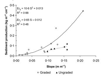
**Figure 9.** Relationship between mean sediment production – normalized by precipitation – and average segment slope (S) for graded  $(Er_g)$  and ungraded  $(Er_u)$  road segments. Solid black line is for graded road segments and dashed line is for ungraded road segments.
