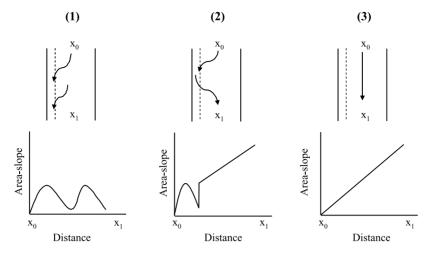
**Figure 3.** Sketches showing the three main drainage patterns of unpaved roads on St John and how this affects the product of road surface area and segment slope: (1) insloped with irregular cross-slope drainage; (2) insloped with a blocked inside ditch; and (3) no effective cross-slope drainage. Dashed lines indicates the inside edge of the ditch.
