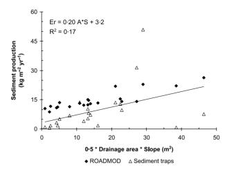
**Figure 12.** Relationship between the annual sediment production rates (Er) measured in this study using sediment traps and the predicted sediment production values using ROADMOD and one-half of the area  $\times$  slope values from Table II. Regression line is for the sediment trap data.
