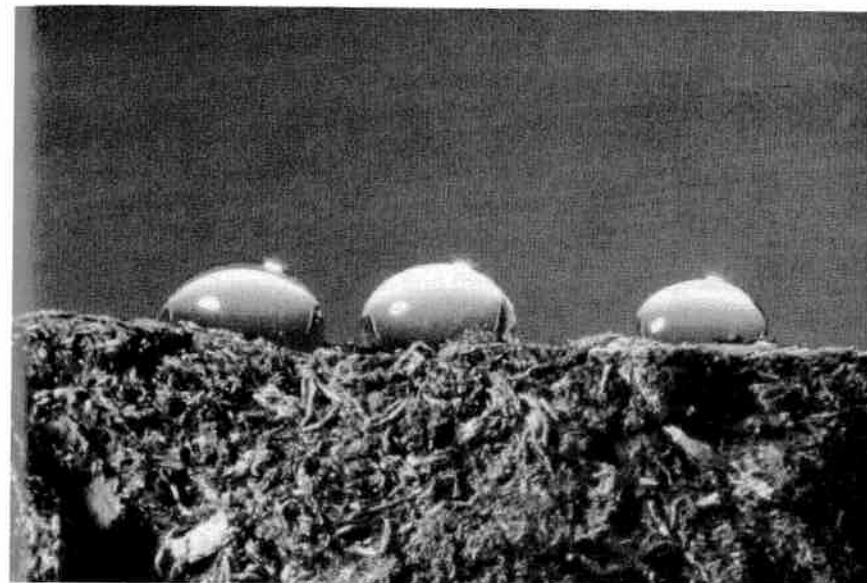
Fig. 1 Water drops resting on a highly repellent organic-rich soil (photo by Erik van den Elsen).
