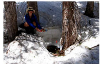
Jill Baron prepares to extract water from a soil lysimeter, a sampling device that captures soil water.
